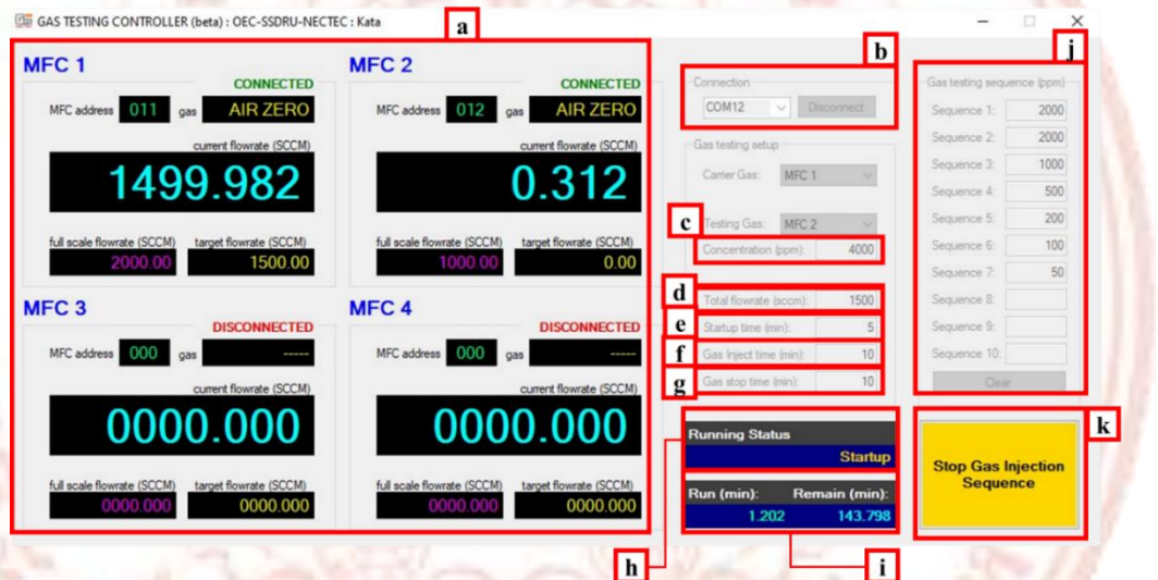
FIGURE 3 -9 Gas testing Controller (beta) Lab-View control program
