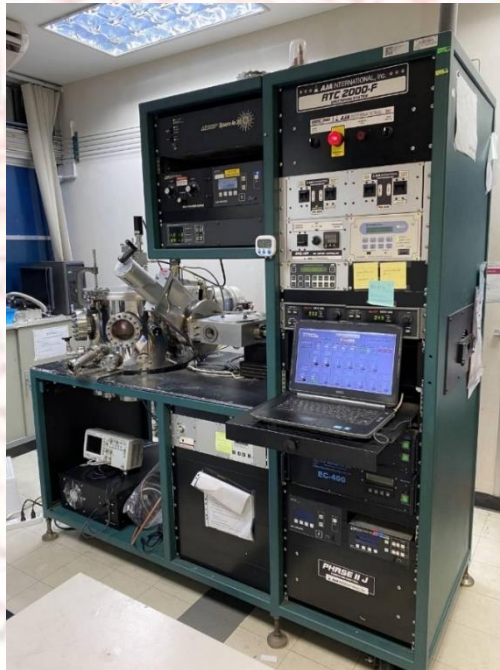
FIGURE 3 -1 (a) The schematic of DC, DC pulsed, and RF magnetron sputter deposition system (b) AJA International, Inc. (ATC 2000-F) at The Optical Thin Film Laboratory, National Electronics and Computer Technology Center (NECTEC)
