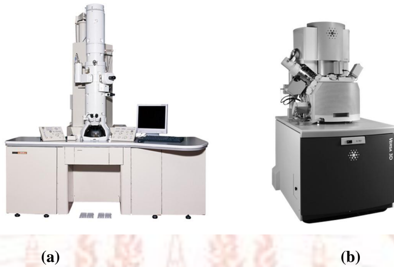
FIGURE 3 -6 (a) High-resolution transmission electron microscope (TEM, JEOL JEM-2010) and (right) field-emission electron microscope/focused ion beam (FE-SEM/FIB, FEI Versa 3D dual beam).
