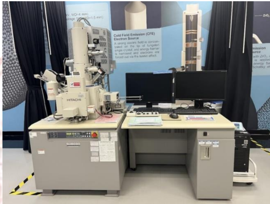
FIGURE 3 -5 The field-emission scanning electron microscope (FE-SEM; SU8030) used to analyze the morphology of thin film
